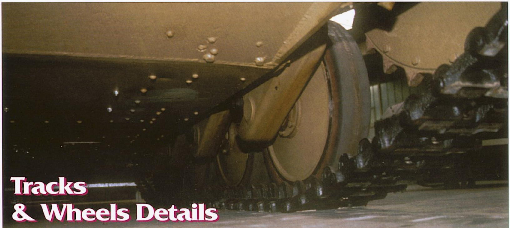
View of the vehicle underside. Note the original tracks and running wheels. Width of the track was 300 mm, with a full track weight on each side of 385 Kg. Note the rubber rims on all road wheels.
