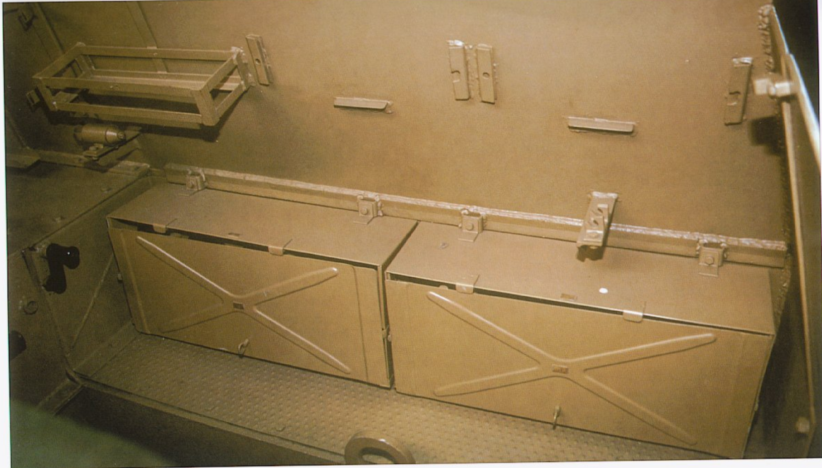
Upper photo - Two ammunition boxes for powder charges, and above are welded frames on the side for stowage boxes. Lower drawings - Open ammunition boxes for powder charges. Each box held eight powder charges.
