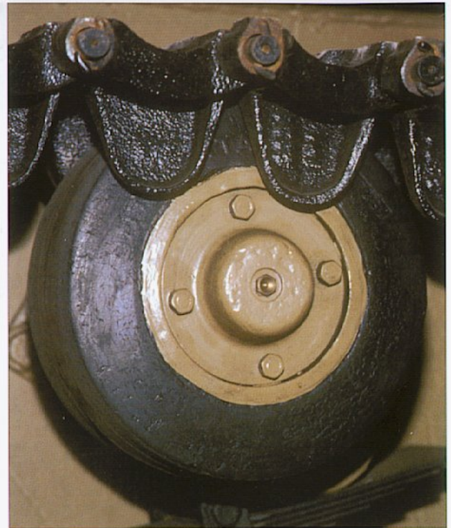
View of the vehicle underside. Note the original tracks and running wheels. Width of the track was 300 mm, with a full track weight on each side of 385 Kg. Note the rubber rims on all road wheels.
