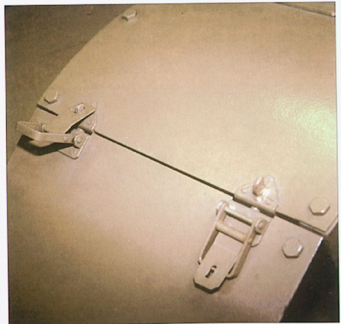
Details of fenders with empty brackets for tools. Note the engine louvers and folding mudguard flap.
